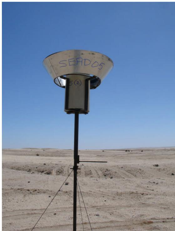
Figure 1: ASTM 1739-98 installation.
