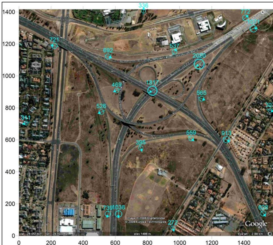
Figure 1. Receptor locations for Buccleuch Intersection simulations. The values represent maximum NO<sub>x</sub> concentrations ( $\mu\text{g}/\text{m}^3$ ) for the base case (i.e. 2006 fuel and 2006 parc split). The vector represents the wind direction resulting in the highest concentrations at the receptor.
